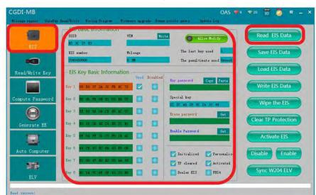
Connect CGDI MB tool to the vehicle via the OBD port, then read the EIS data.
