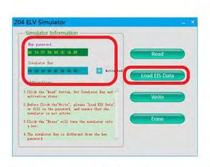
Load the EIS data just saved and check whether the key password is correct
